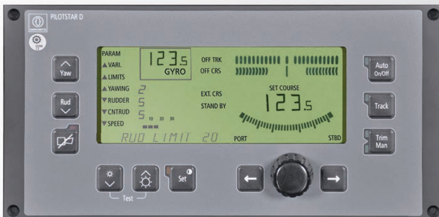
The operator unit provides clear indication of all necessary data and ease of use
